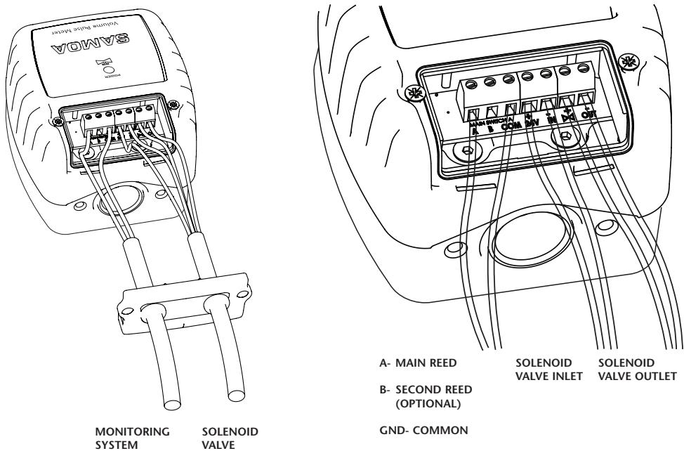
The electronic board LED allows quickly display of the open (LED on) or closed (LED off) state of the solenoid valve, if that is installed on the line.
