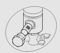
3 REMOVE THE FILTER BOLT
